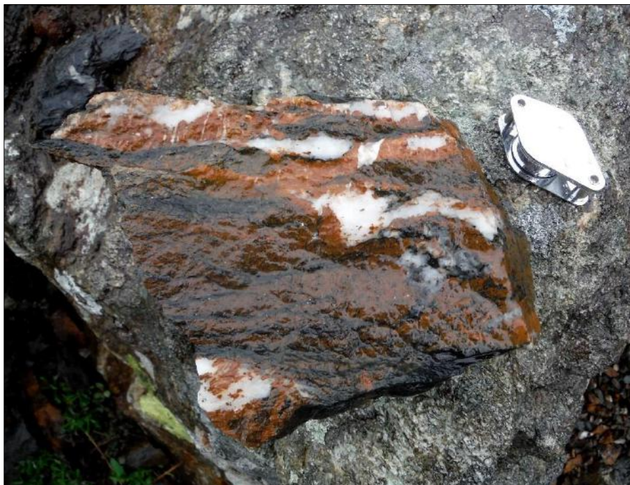
Figure 3-15 Fragment of quartz vein material from Oscarsgangen showing ribbons of host rock, abundant ankerite and disseminated pyrite (SRK ES, 2018)
