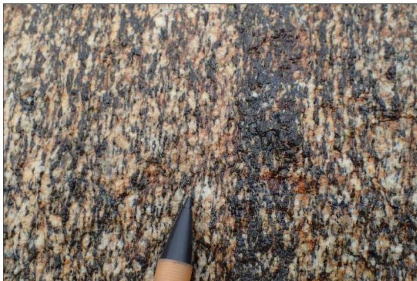
Figure 4-10 Close-up photo of the layering and foliation in a modally layered gabbro-norite (SRK ES, 2018)
