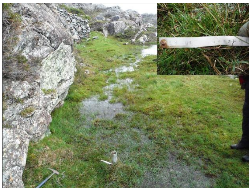
Figure 3-20 Apparent drillhole collar from an unknown programme discovered about 200 m NE of the Harald Haarfagres mine (SRK ES, 2018)
